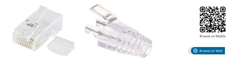
NEXCONEC<sup>®</sup> Category 6A RJ45 plug exceeds the transmission line performance requirements of IEC and TIA for CLASS EA/Category 6A systems. Each Category 6A RJ45 plug supports all applications designed for CLASS EA networks, as defined within ISO/IEC 11801 (2nd Edition):2010 including 10GBASE-T (10 Gigabit Ethernet), 2G FCBASE-T, 4G FCBASE-T and 1000BASE-T (Gigabit Ethernet.
