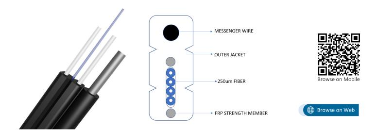
NEXCONEC FTTH Drop Cable is made of 1 to 4, 250µm individually colored optical fibers with fiber reinforced strength members, steel wire which also acts as messenger wire and UV resistant Low Smoke Zero Halogen (LSZH) or PE jacket. The steel wire provides additional strength suitable for aerial applications.
