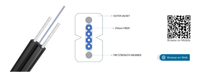
NEXCONEC® FTTH Drop Cable is all dielectric drop cable consisting of 1 to 4, 250µm individually colored optical fibers with Fiber Reinforced Plastic (FRP) strength members and UV resistant Low Smoke Zero Halogen (LSZH) or PE jacket.
