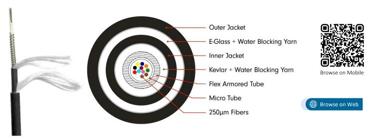
NEXCONEC® Indoor & Outdoor Microcore Flex Armored cable contains 12 fibers of 250µm fibers in a micro tube, which is accommodated in the helical flex armored tube, then with E-glass, Kevlar and water blocking yarn added in the cable to make ideal use in the indoor/outdoor environment where anti-rodent is needed.
