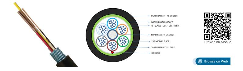
NEXCONEC<sup>®</sup> Corrugated Steel Tube Armored Multi Loose Tube is made of multiple single gel filled PBT tubes and each tube consists of 12, 250µm optical fibers, the tubes are surrounded with longitudinally applied E-glass non-metallic strength members, Corrugated Steel Tube (CST) armor and UV resistant LSZH or HDPE jacket.
