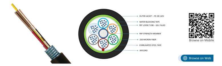
NEXCONEC Corrugated Steel Tube Armored Multi Loose Tube is made of multiple single gel filled PBT tubes and each tube consists of 12, 250µm optical fibers, the tubes are surrounded with longitudinally applied E-glass non-metallic strength members, Corrugated Steel Tube (CST) armor and UV resistant LSZH or HDPE jacket.
