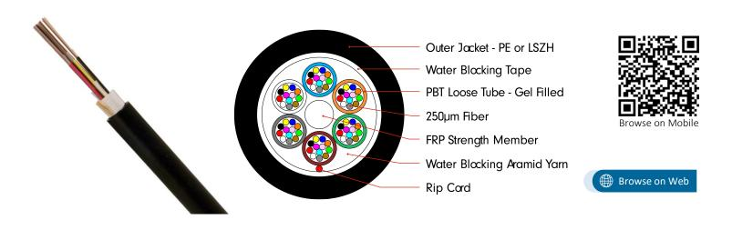
NEXCONEC Multi Loose Tube is made of multiple single gel filled PBT tubes and each tube consists of 12,  $250\mu m$  optical fibers, the tubes are surrounded with longitudinally applied E-glass non-metallic strength members, UV resistant LSZH or HDPE jacket.
