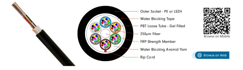
NEXCONEC<sup>®</sup> Multi Loose Tube is made of multiple single gel filled PBT tubes and each tube consists of 12, 250µm optical fibers, the tubes are surrounded with longitudinally applied E-glass non-metallic strength members, UV resistant LSZH or HDPE jacket.
