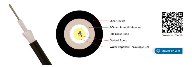
NEXCONEC Single Loose Tube is made of single gel filled PBT tube that consists of 2 to 24, 250µm optical fibers, the tube is surrounded with longitudinally applied E-glass non-metallic strength members, UV resistant LSZH or HDPE jacket.
