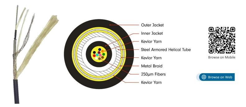
NEXCONEC Outdoor Single Loose Tube Flex Armored Fiber Cable is made of a subunit which consists up to 12 250µm fibers and with aramid strength member. Then in the helical tube and surrounded with metal braiding and PU jacket for high crush resistance for outdoor application.
